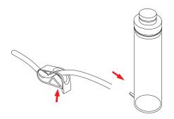
**Step 3:** Connect the other end of the tube to the fuel cell lower fuel inlet. Make sure the connection is tight. Cut a 10cm long tube and connect it to the other outlet of the fuel cell (the remaining nozzle).
