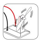
Note: Once the fan stops rotating, open the clamp to purge some solution out of the fuel cell. Wait for 5-10 minutes with the cable disconnected from the fan module, the fan should start rotating by itself once connected. Make sure you repeat the waiting period of 5-10 minutes after each purging. Since the reaction is slow, the fan can run for up to several hours without puraina.
