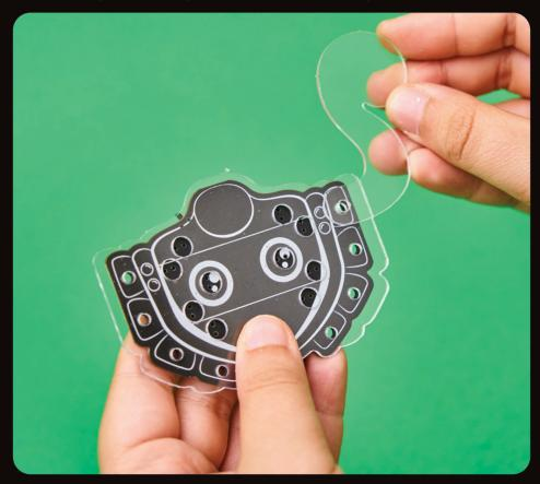
Put the bolts on the front and the standoffs in the back.
