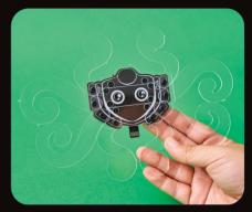
Next, take the coin battery and place it on the backside (make sure the + symbol on the battery matches the + sign on the board - front and up).
