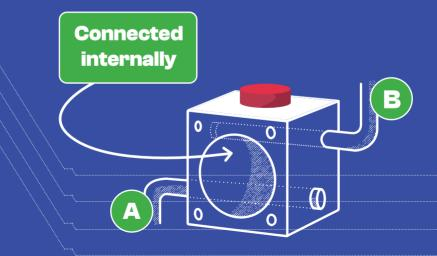
Because the internal contact within the pushbutton connects while the button is pressed, the electrical circuit is closed, and current can flow. When we release the pushbutton, the electrical circuit opens, and the current no longer flows.
