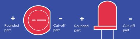
You can recognize the polarity by the shapes of the sides of the diode. The positive side is rounded and called the **anode**, while the negative side is flat and called the **cathode**. Electrical energy always travels from the anode to the cathode, never vice versa.
