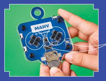
When it comes to Marv's LEDs, it's super easy. You'll find the **polarity** indicated by **plus and minus marks**. So, when you turn on Marv and start adding LEDs, just be sure to pay attention to their polarity as you connect them. Look for the cut-off (-) and rounded (+) parts marked on the LED – they'll tell you all you need to know.
