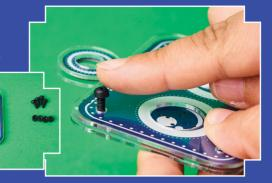
Here's how you do it: **put the bolts in from the front and add the standoffs onto the back**.
